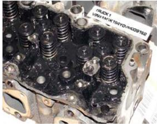
Figure 1.5 - B20 valve deck sludge accumulation according to Richard Fraer et.al. [6]
