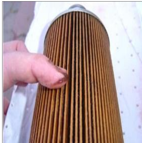
Figure 1.4 - Plugged B20 fuel filter in accordance with Kennteh Proc et.al. [5]
